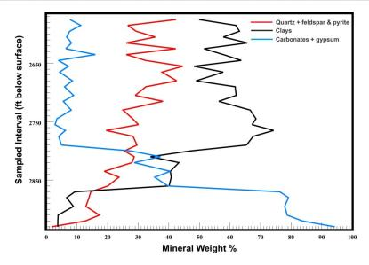
XRD Analysis of No. 1-3613 Rowe-Grube Unit Well, API# 3408926065, Licking Co., OH
