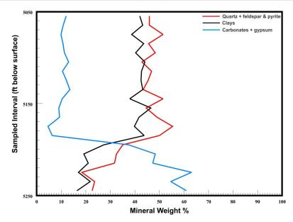
XRD Analysis of No. C-1 Commonwealth of PA Tract 163 Well, API# 3710320003, Pike Co., PA
