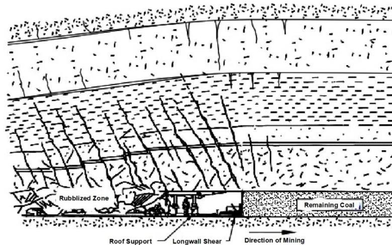
**Figure 5: Cross section of typical longwall face with resultant rubblization of overlying strata after mining, adapted from Mine Subsidence Consultants (2007). Note the rubblization of overlying strata behind the roof supports.**
