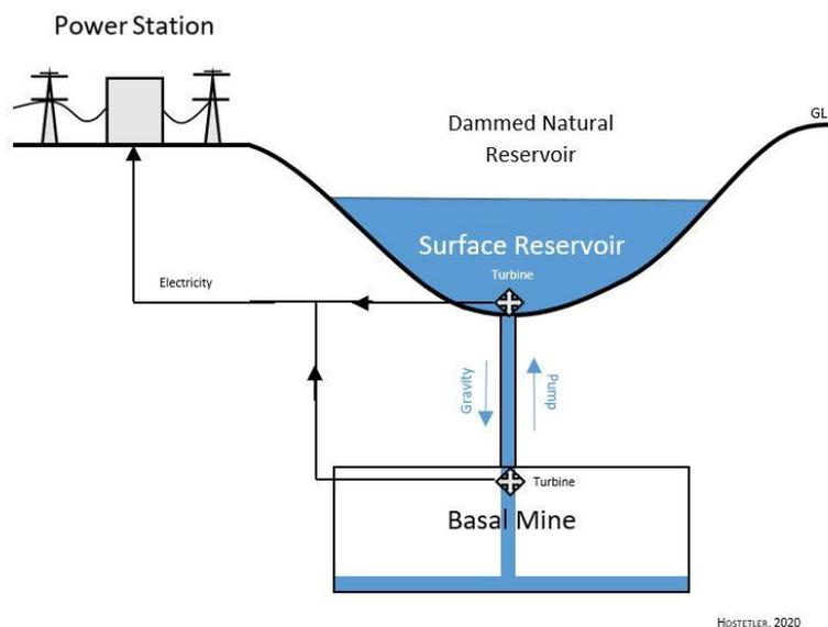
**Figure 3: Simple schematic diagram of a mine pump storage System utilizing an upper surface reservoir with a lower mine.**
