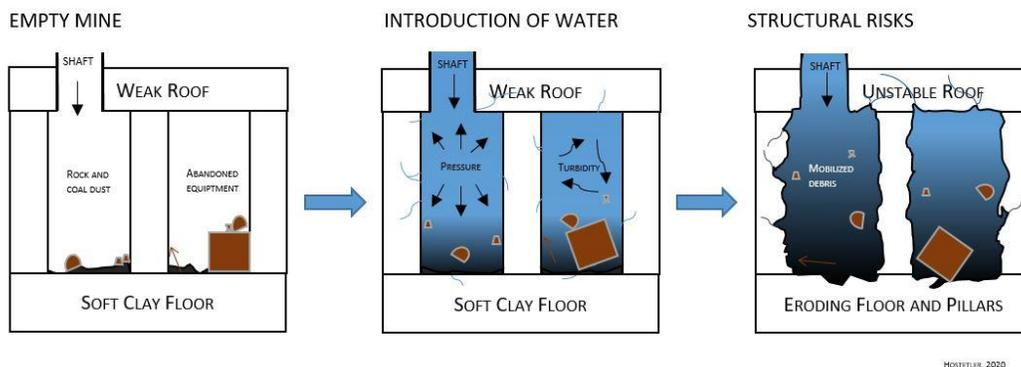
**Figure 2. Rapid infilling of mine voids during daily pumping cycles will cause tremendous amounts of erosion within the lower mine. Displaced debris could hinder water flow through the mine or clog pumps.**
