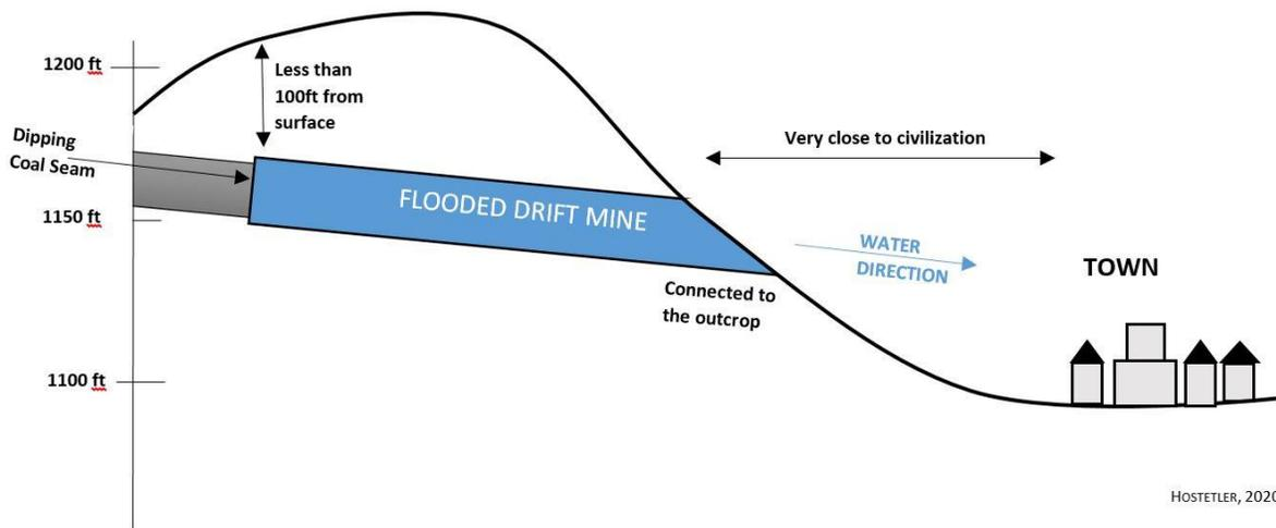
**Figure 6: Diagram showing a down dip mine and the difficulty of adequately sealing the mine void.**
