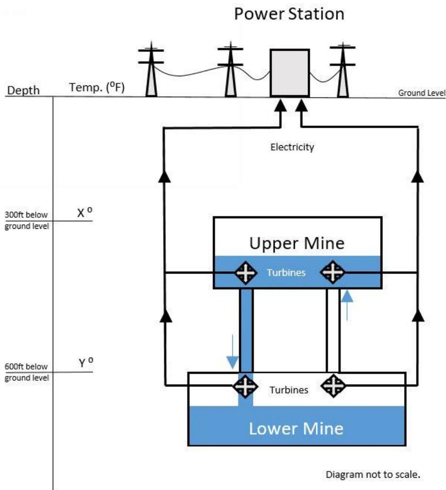
**Figure 1: Simple schematic diagram of a mine pump storage system utilizing 2 mines separated vertically by at least 100 feet. Mines do not necessarily need to be stacked directly above one another. A lateral offset is also acceptable.**
