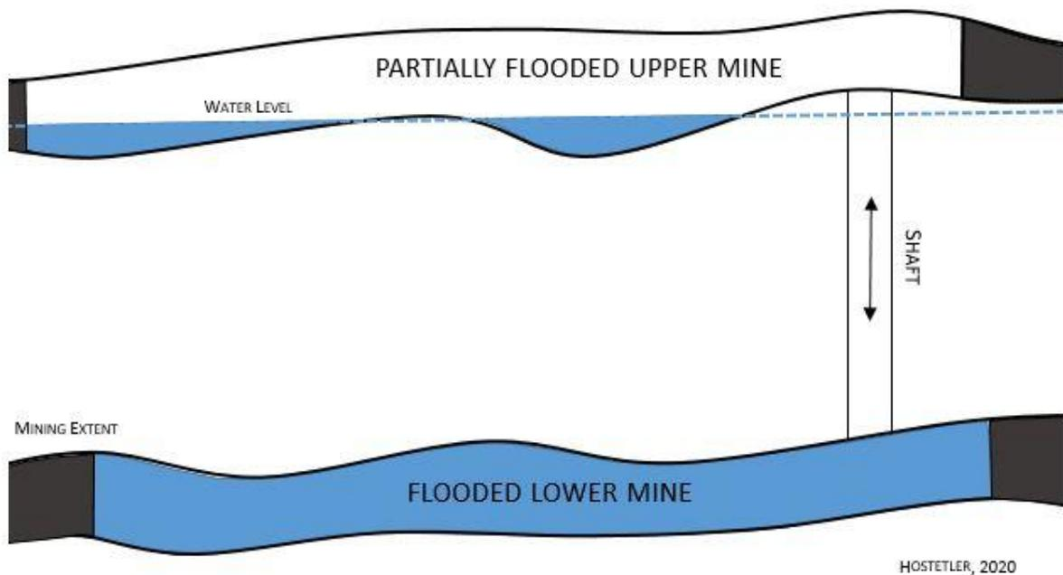
**Figure 7. Structural undulations will cause high spots in mines possibly impeding drainage.**
