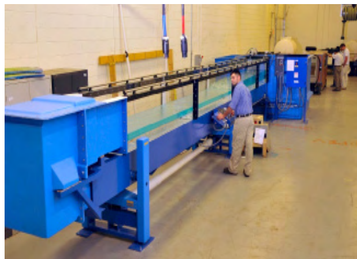
Figure 27 (left). Research level flume table. Source: http://tpapanicolaou.engr.utk.edu/consulting-facilities/
