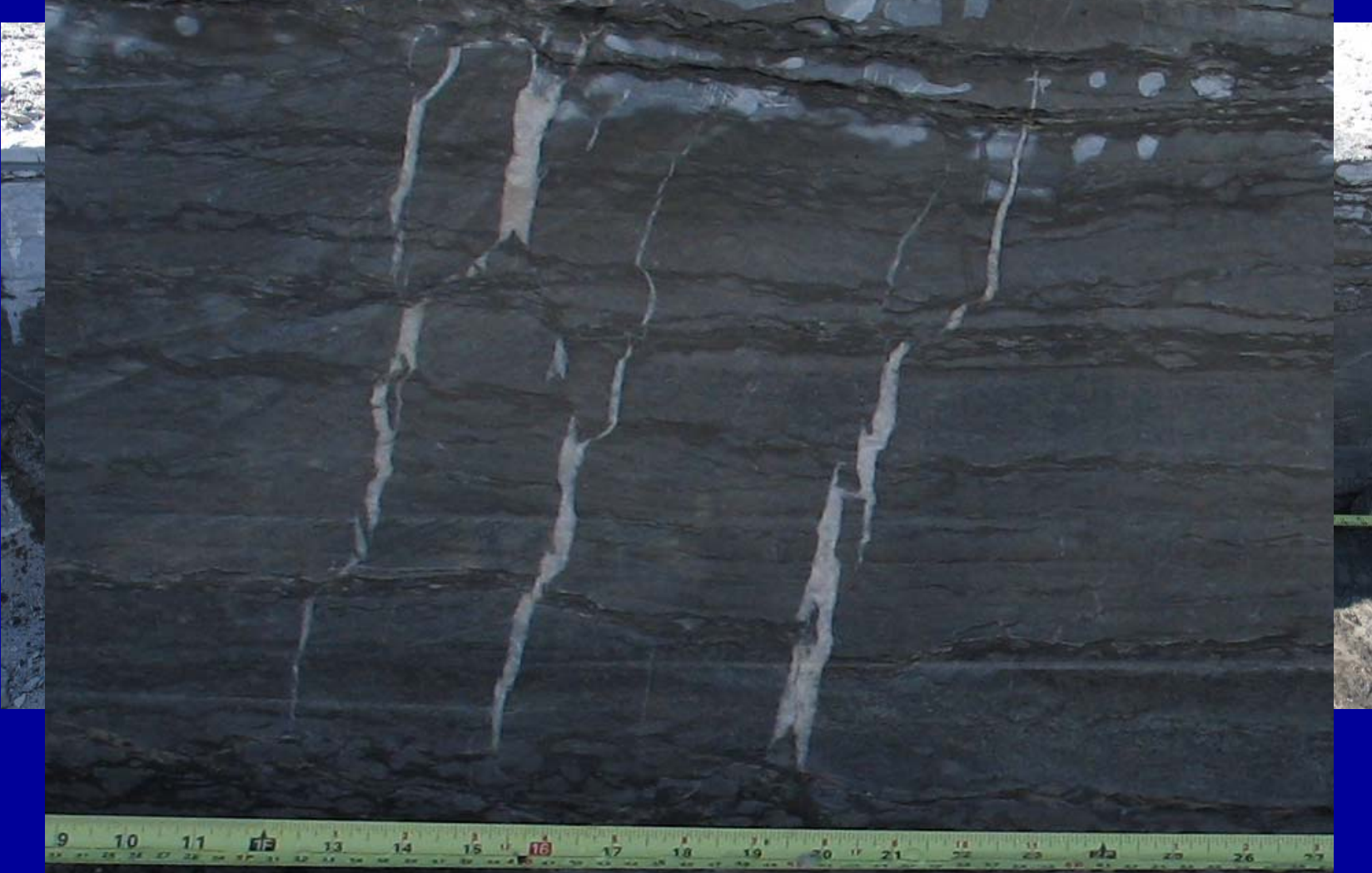
Fractures dip away from the dolomite body and are plugged with calcite on the south side
