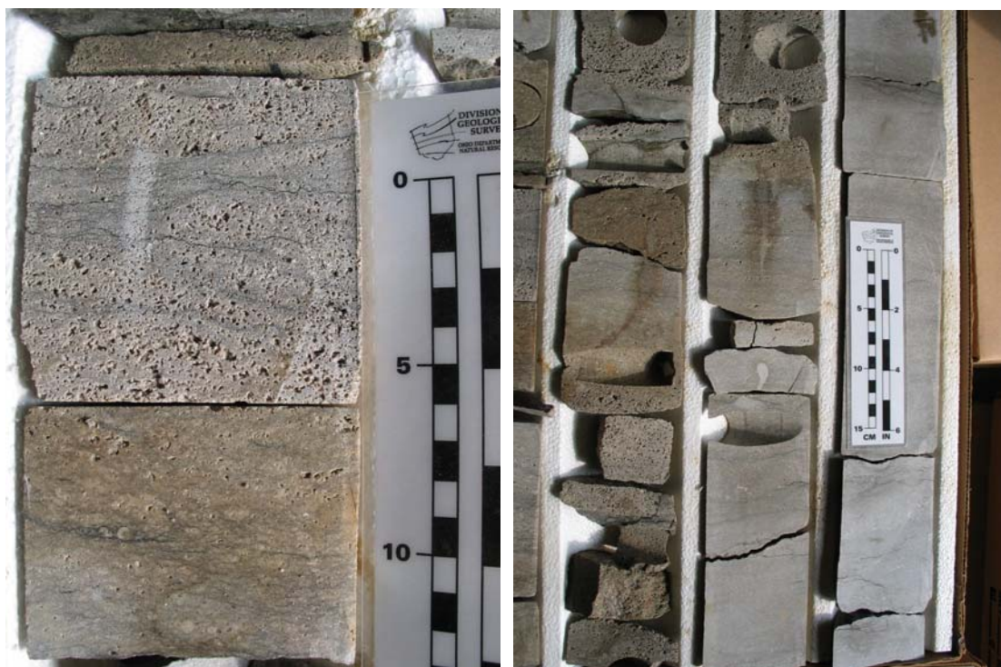
Figure 49. Facies dolomite core from NW Ohio with coarse, porous matrix dolomite that was probably a grainstone prior to dolomitization. Scale is in cm.
