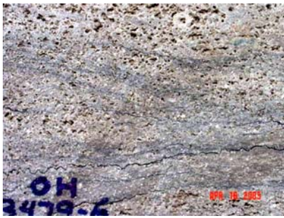
Figure 31. Dolograins from Trenton Group reservoirs in northwest Ohio. A. Dolograins with recognizable depositional texture. The rock consists of cross-bedded, coarse-grained crinoid-bryozoan grainstone interbedded with stylolitic dolomudstone/dolowackestone. These cyclic lithologies consist of shoaling-upward, grainstone-capped subtidal parasequences. Note the large crinoid allochem, which is mimetic planar-s to nonplanar-a (transitional) dolomite (also see Figure 32). The visible porosity consists mostly of small vugs, 0.5 to 4 mm in diameter, and molds. (OH 3479, Hancock Co., Palladin Enterprises, Anderson well, 1337.8 ft.). B. Interpreted dolograins without recognizable depositional texture. Dolomitization has obliterated all of this rock's primary and earlier diagenetic fabrics. The interpretation of this sample as a former grainstone is based on the presence of allochem ghosts, and both mimetic and non-mimetic replacement textures observed in thin section (Figure 33). (OH 3267, Auglaize Co. Meridian, Bousher #1 well, 1174 ft.).
